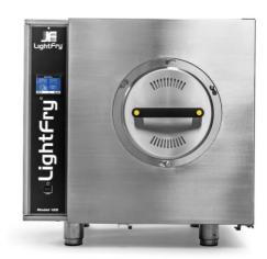
Dimensions: W693 x H695 (incl. chimney 711) x D645 mm (incl. handle 690 mm) Net weight: 100kg Electrical connection: 3x400V + N, 50–60 Hz, 16 kW Drainage connection: 25 mm Fresh water connection: 19 mm Extract air: Extractor hood or customised Lightfry hood (see regulations) Capacity: Up to 22 kg per hour. From 200g to 2.5kg batch. Example: 600 grams of French fries(6x6mm) in 3:50 - 4:20 minutes Material: Stainless steel oven and casing
