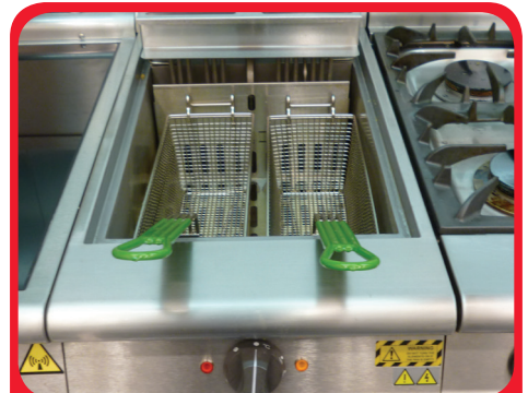
Step 9 - Close drain valve. Replace fry plate and baskets.
