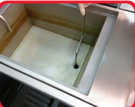
Step 7 - Using the included tool, ensure drain valve is clear of any debris.
