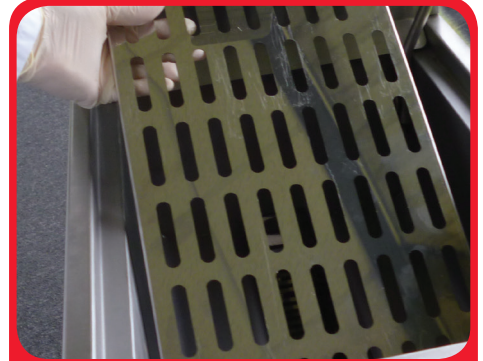
Step 3 - Remove baskets and fish plate. Wipe clean with damp cloth. Dry thoroughly.
