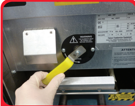
Step 2 - Drain oil into oil bucket.
