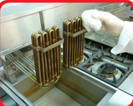
Step 4 - Remove elements from pan and clean with damp cloth. Dry thoroughly.
