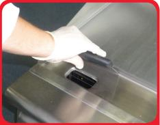
Step 3 - Drain any liquid fat present into the grease jug.
